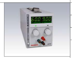
The XPD can be combined in a mix-and-match configuration with the quarter-rack 300-watt HPD series and 60-watt XT series. Each unit features zero voltage "soft switching" to virtually eliminate switching transients. This switching technology contributes to high efficiency, low noise, and high reliability. The XPD series also features power factor correction (PFC) technology to enable low current draw and to greatly reduce generation of input current harmonics.
